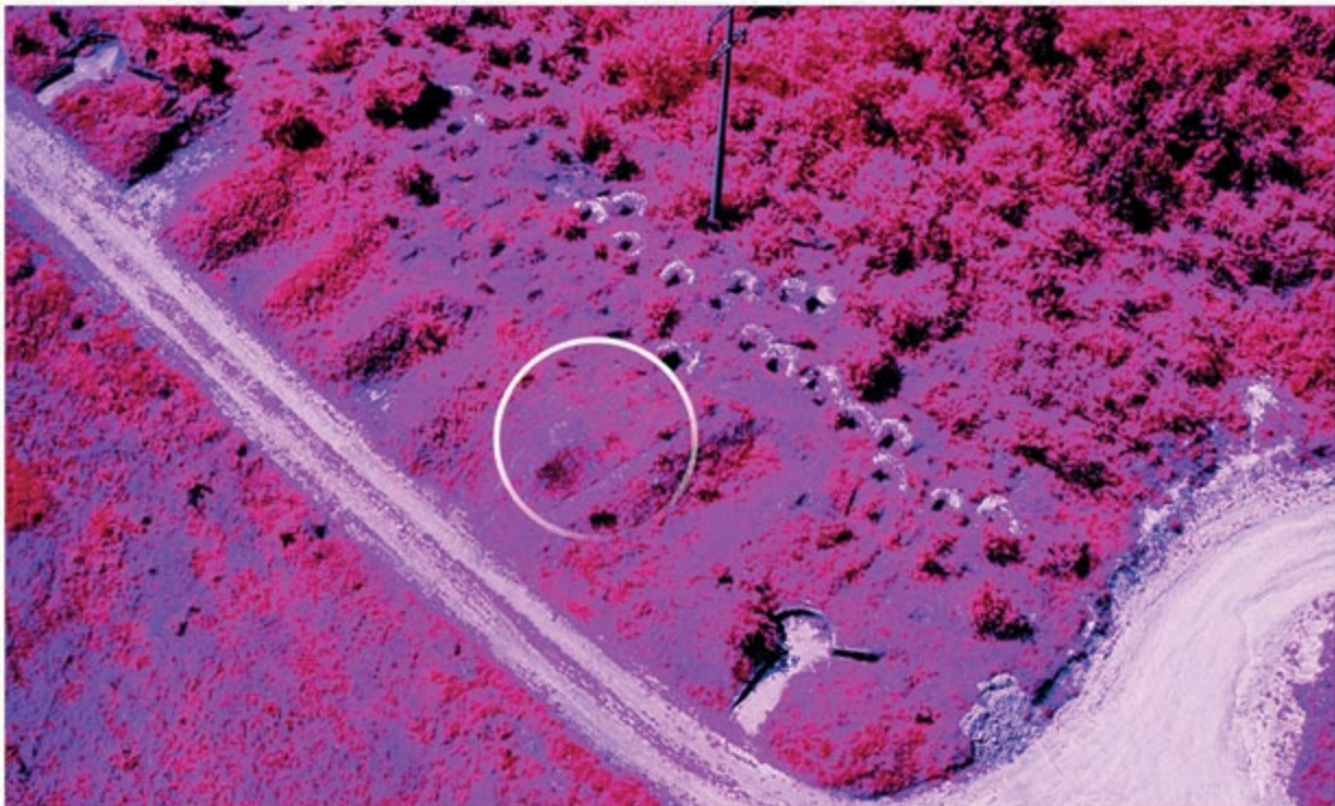
Aerial IR color photography of vehicle camouflaged with MD99-net
